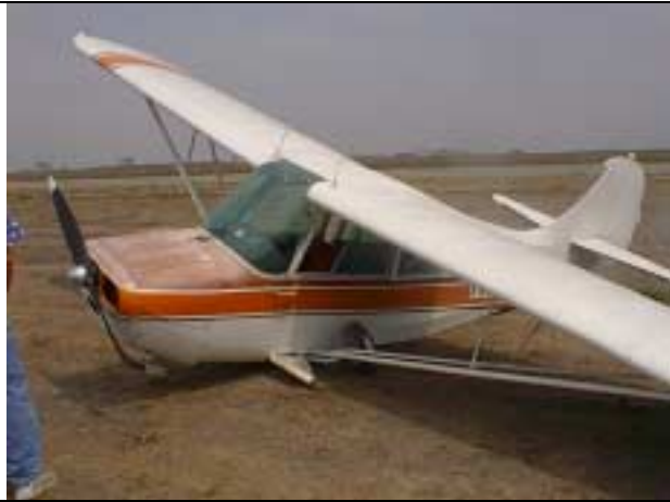
The Flying J Champ had a mishap during our monthly meeting; went thru a ditch that broke the left gear.
