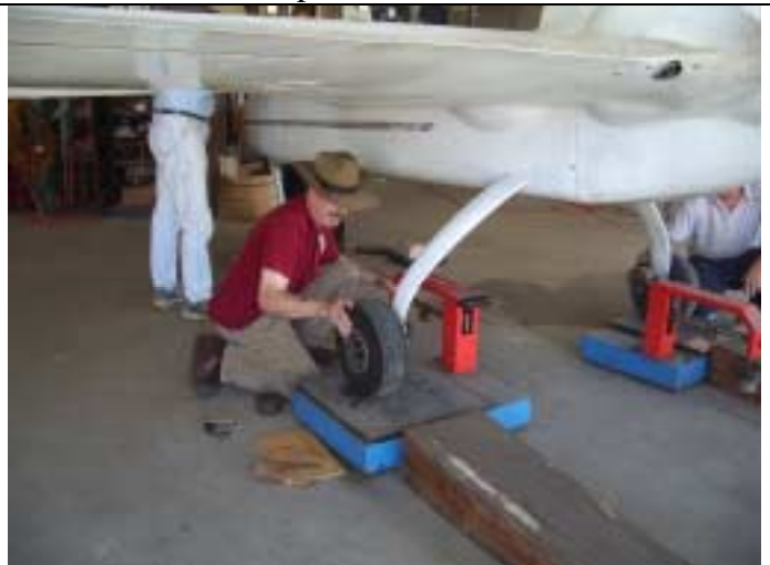
Dan Patch preparing to weigh an EZ
