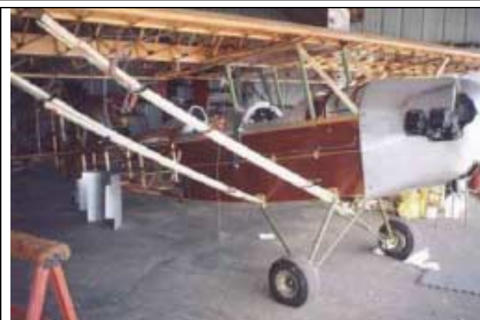
Gene's Pietenpol with temporary lift struts in place.
