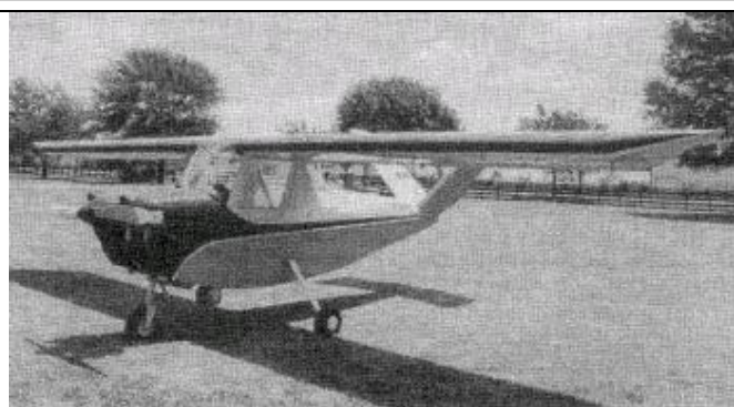
Honey Bee – Single place, high wing, all metal, 65HP Cont. cruise 106mph, 900 fpm, EW 639, Gross 960. Sport Ready. 100 Oct. valves & carburetor, chrome cyls, entire airframe primed on inside. Shielded ignition. Prototype got type cert 4A11 in 1953. $17,000, pics on request. 281-342-1801
